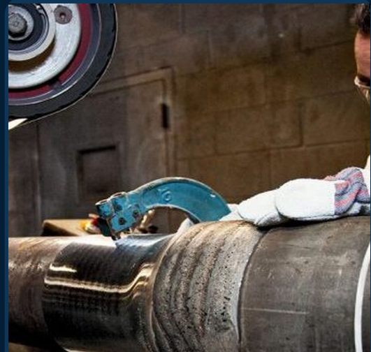
Drill-pipe thread and dimensional inspection
